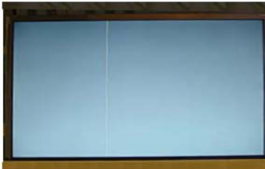
Vertical Line Source TAB IC Defect
