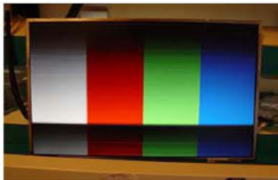
Horizontal Block Gate TAB IC Defect
