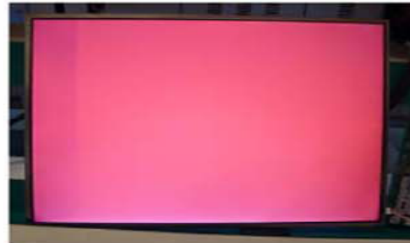
Vertical Block Source TAB IC Defect
