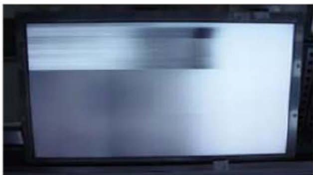
Horizontal Block Gate TAB IC Defect
